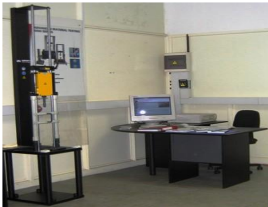
Figura 14. Echipament integrat INSTRON - Dynatup Drop Weight Impact Test Machine Model 8200 (sala CF009bis) © 2011-TCM-LTPC
